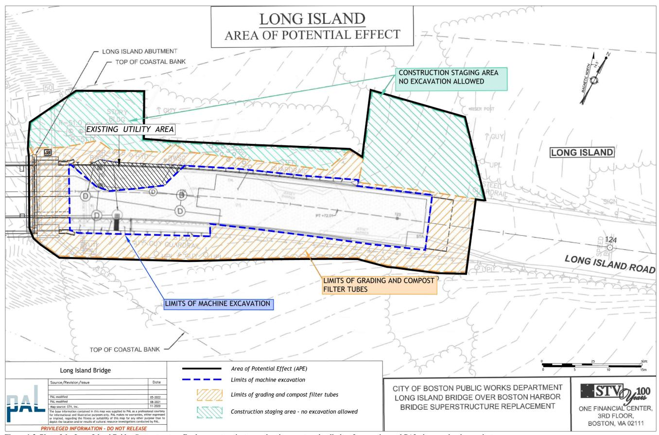
Figure 1-3. Plan of the Long Island Bridge Superstructure Replacement project area showing construction limits of excavation and PAL site examination project area.
