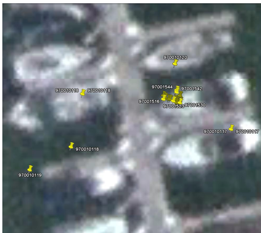
Figure 7: Zooming in further shows the various AIS transmissions detected from the test unit AIS-EPIRB (...117), AIS-SARTs (numbers ...118, 119 & 120) and the cluster of detections from the Class-A unit (...1515 and incrementing to 1544)
