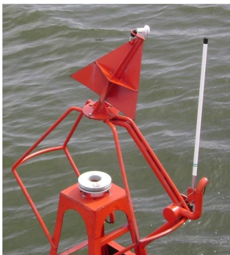
Figure 7 Antenna damage due to collision
