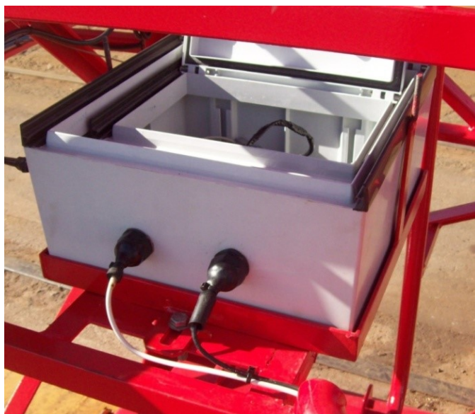
Figure 15 Example of a double enclosure
