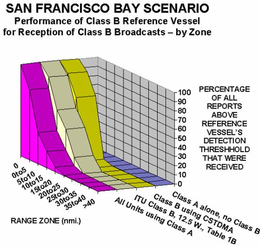
**Percentage of possible Class B receptions that were correctly received aboard reference Class B vessel during indicated simulation scenarios.**
