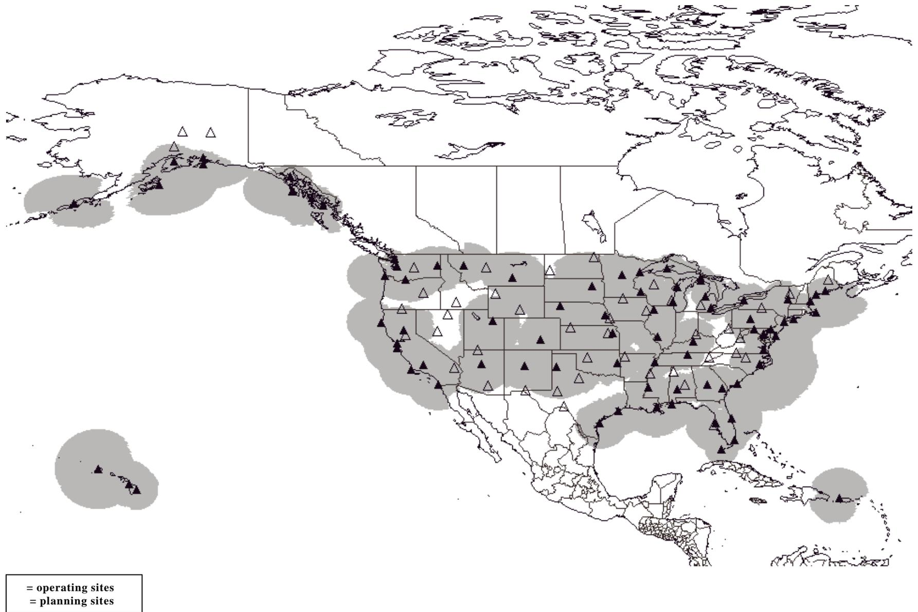
**Figure 3-2. U.S. MF Radiobeacon DGPS Service Coverage**
