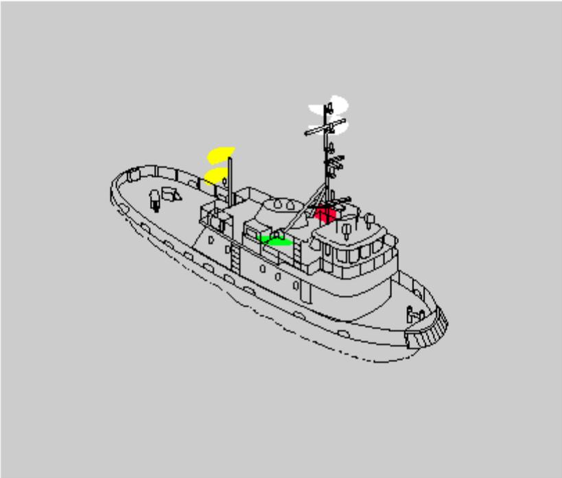
Power-driven vessel pushing ahead or towing alongside—
