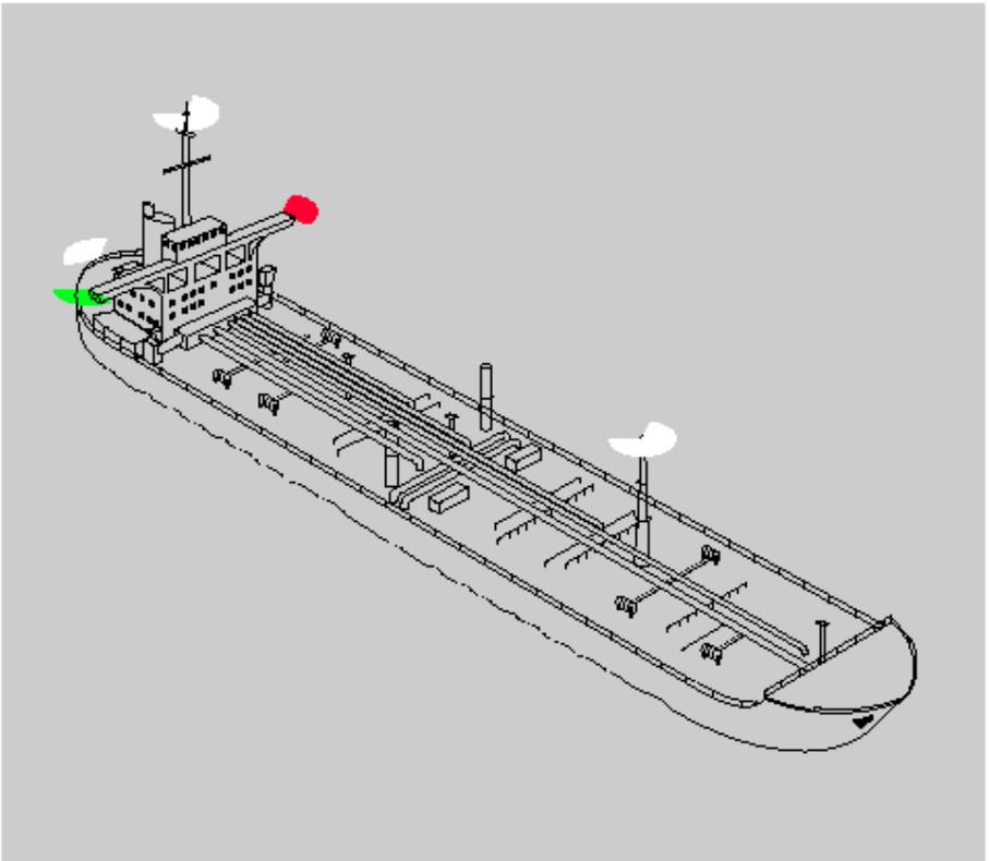
Power-driven vessel underway- 50 meters or greater in length.
