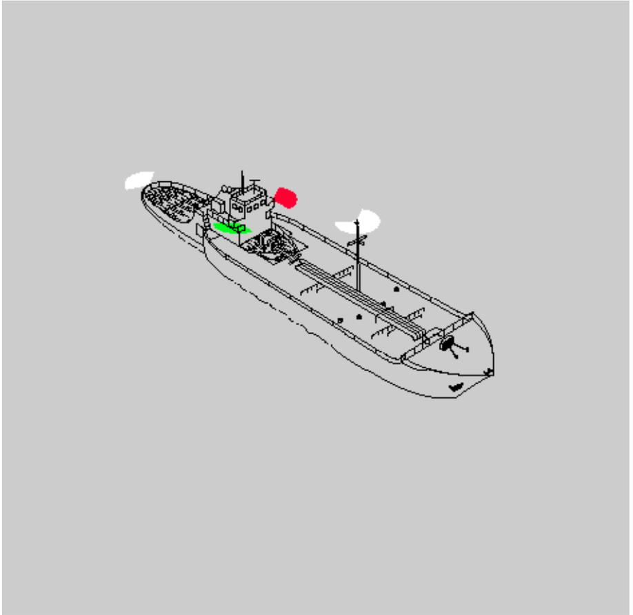
Composite unit underway - less than 50 meters in length.
