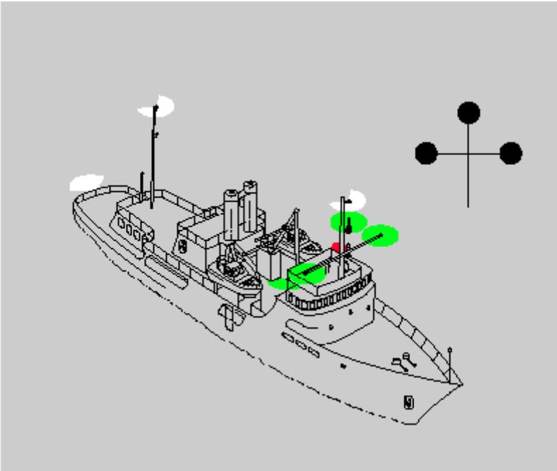
Vessel engaged in mineclearance operations.
