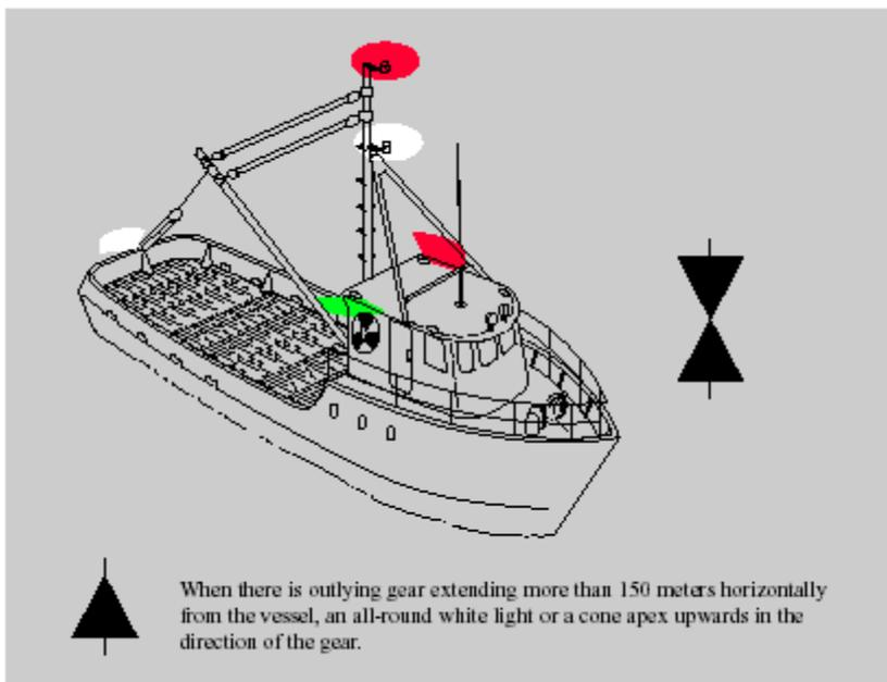
Vessel engaged in fishing other than trawling—making way.
