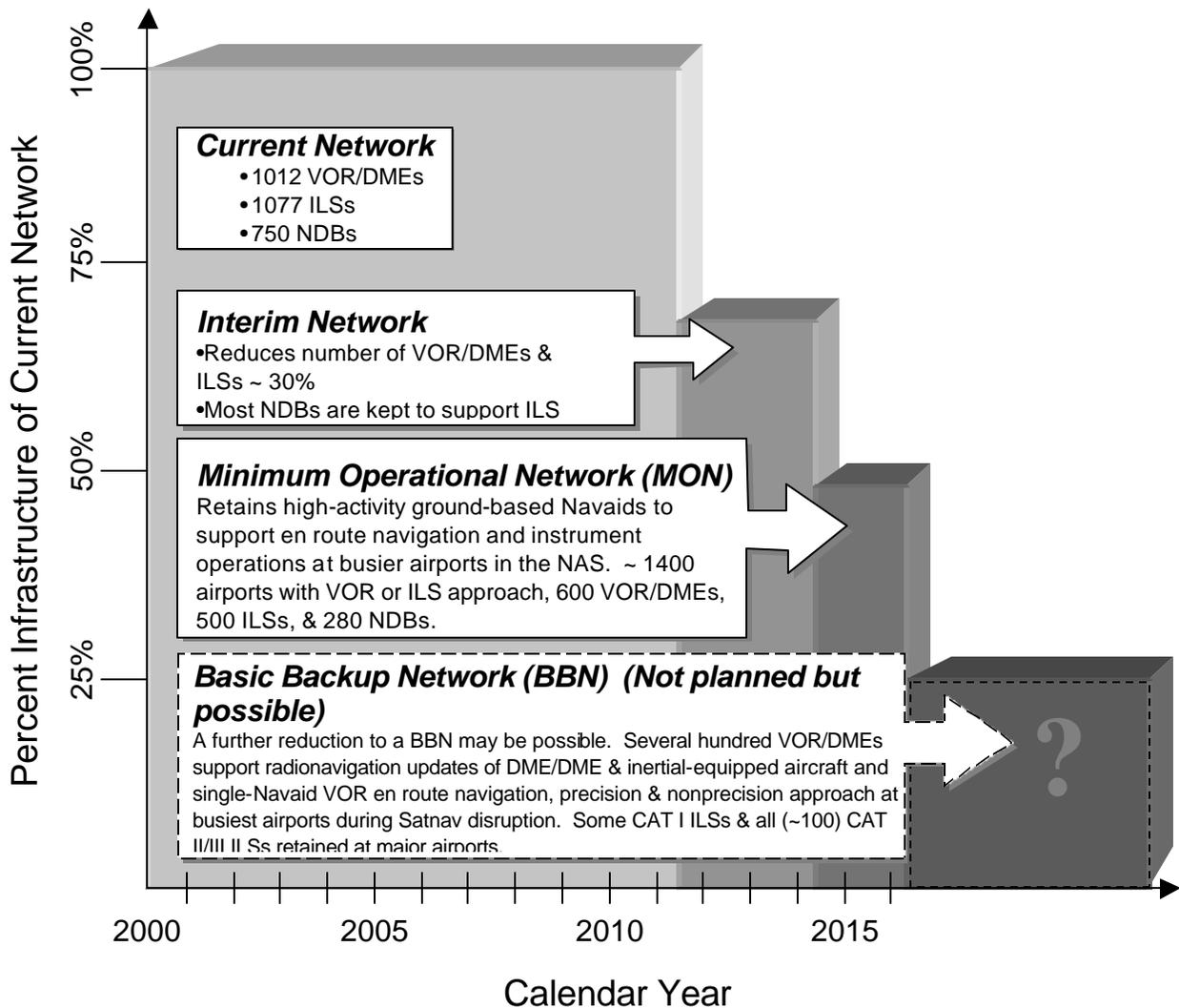
**Figure 3-2. Proposed Civil Aeronautical Navaid Phase-Down Steps**
