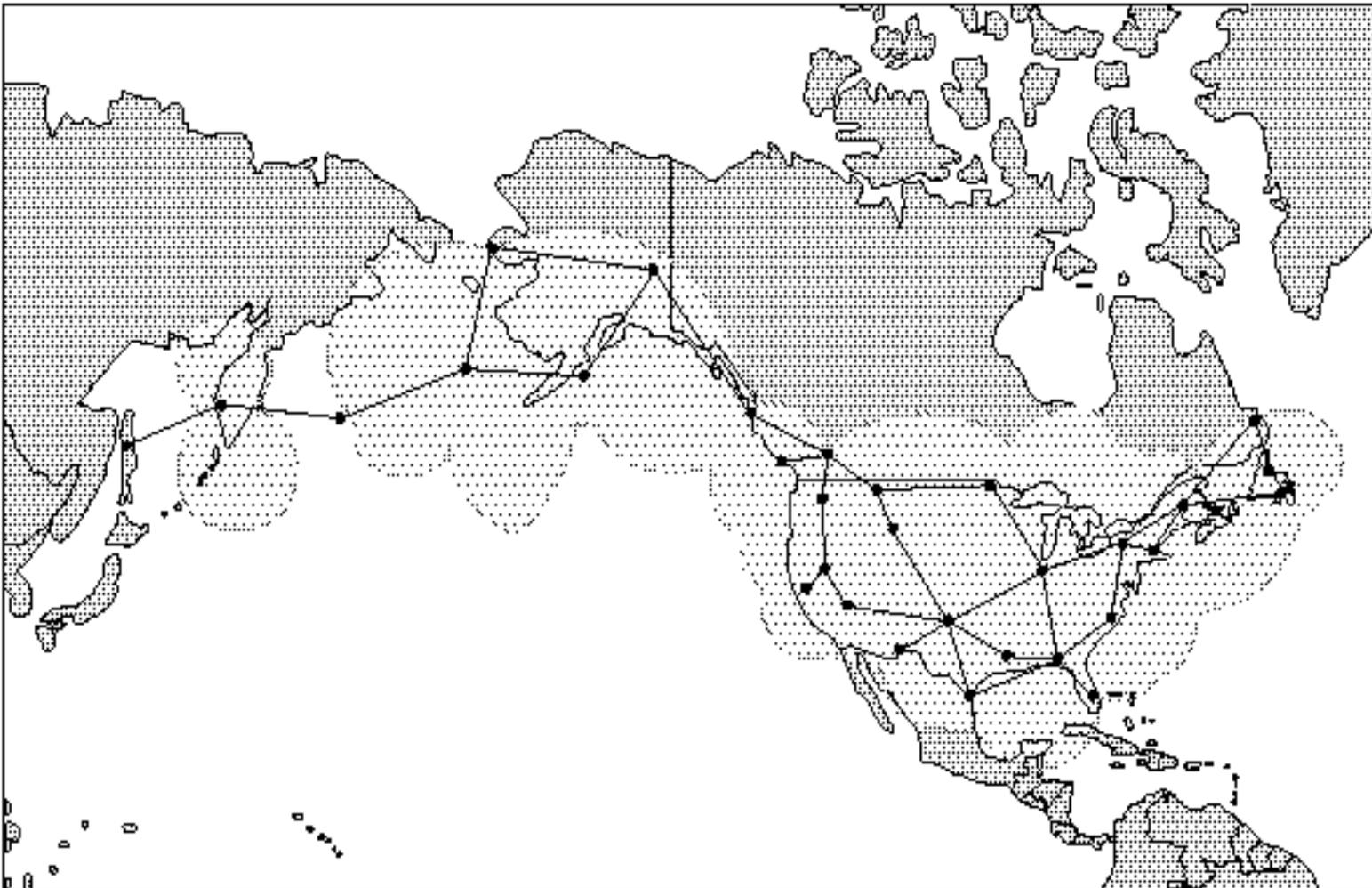
Figure 3-5. Coverage Provided by U.S. or Supported Loran-C Stations
