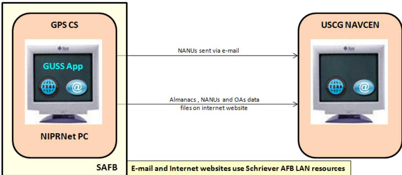
Figure 2 GPS CS to USCG NAVCEN Interface
