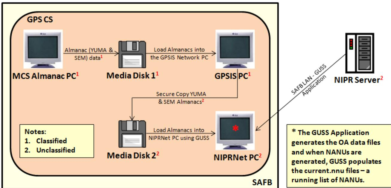
Figure 1 GPS CS to GUSS Interface
