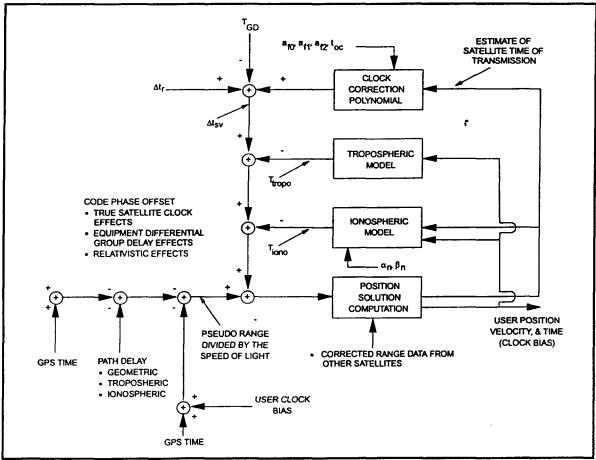
Figure 2-11. Application of Correction Parameters
