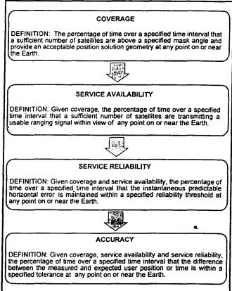
Figure 1-1. GPS Performance Parameters
