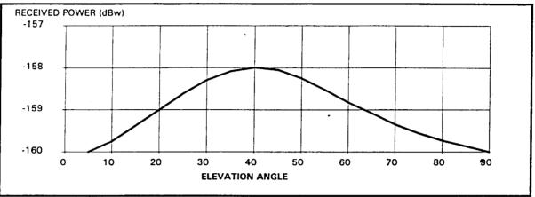
Figure 2-6. User Received Minimum Signal Levels
