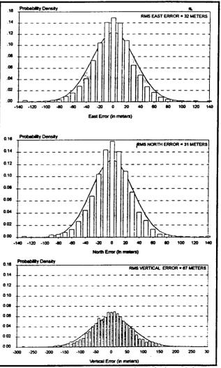
Figure 5-6. SPS Error Distributions in Local Axes
