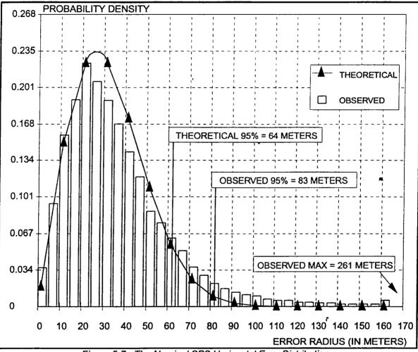
Figure 5-7. The Nominal SPS Horizontal Error Distribution
