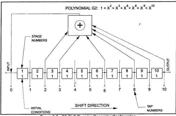
Figure 2-3. G2 Shift Register Generator Configuration
