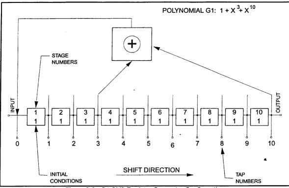
Figure 2-2. G1 Shift Register Generator Configuration
