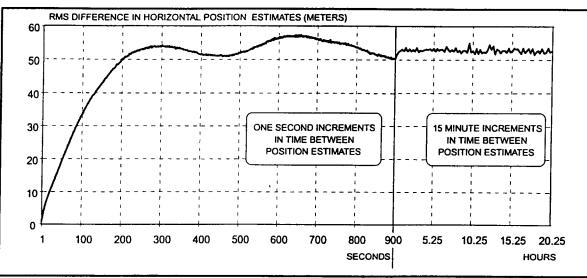
Figure 5-8. Repeatable Accuracy as a Function of Time between Position Estimates
