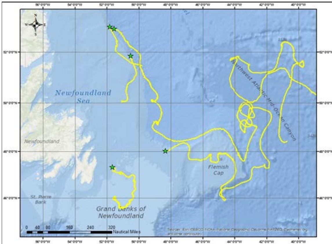
Figure 12. Composite buoy tracks. Green stars indicate Argos-tracked SVP buoy deployment positions. Yellow tracks indicate individual SVP buoy paths.
