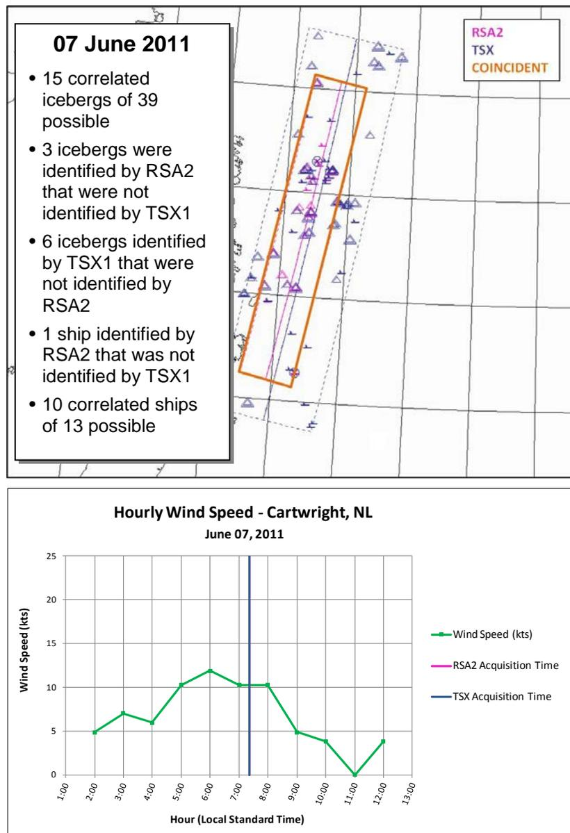
**Figure B-2: Coincident areas and detections for RSA2 and TSX on 07 June 2011 (top) with hourly wind speeds at Cartwright, NL (bottom). (Wind data courtesy of Environment Canada).**
