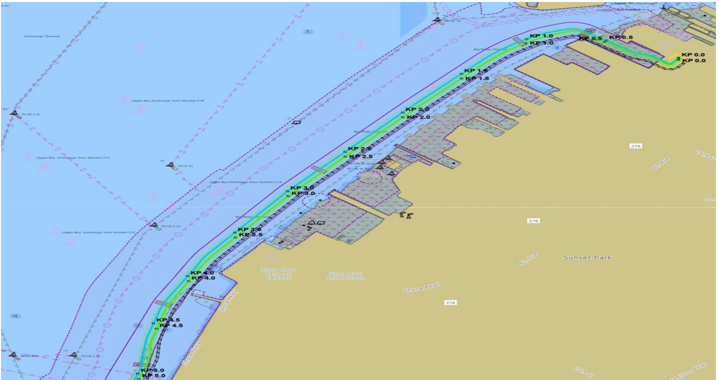
Figure 4: Submarine Export Cable Corridor through Bay Ridge Channel. Marmac 306 may remain stationary for several days at the start (KP0.6) and end (KP5) of this section. The expected time for pre-trenching in this section is 4-5 days for each cable route. The expected time to complete cable installation in this section is 4-5 days for each of the two cables.
