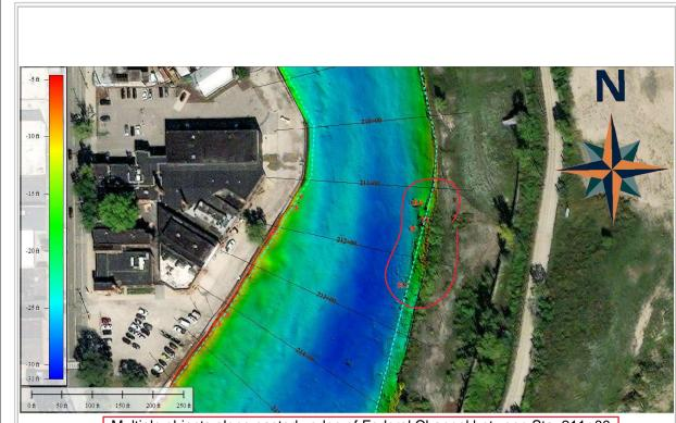
Multiple objects along easterly edge of Federal Channel between Sta. 211+00 & 213+00. Object Depths shown in red. Federal Channel shown in cyan.
