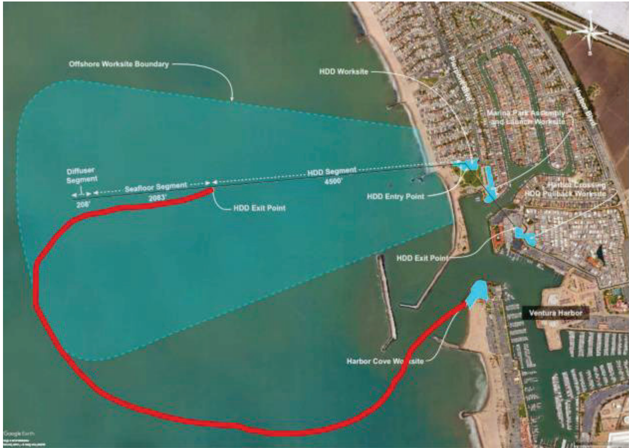
Seafloor Segment HDPE Pipeline pull-out route
