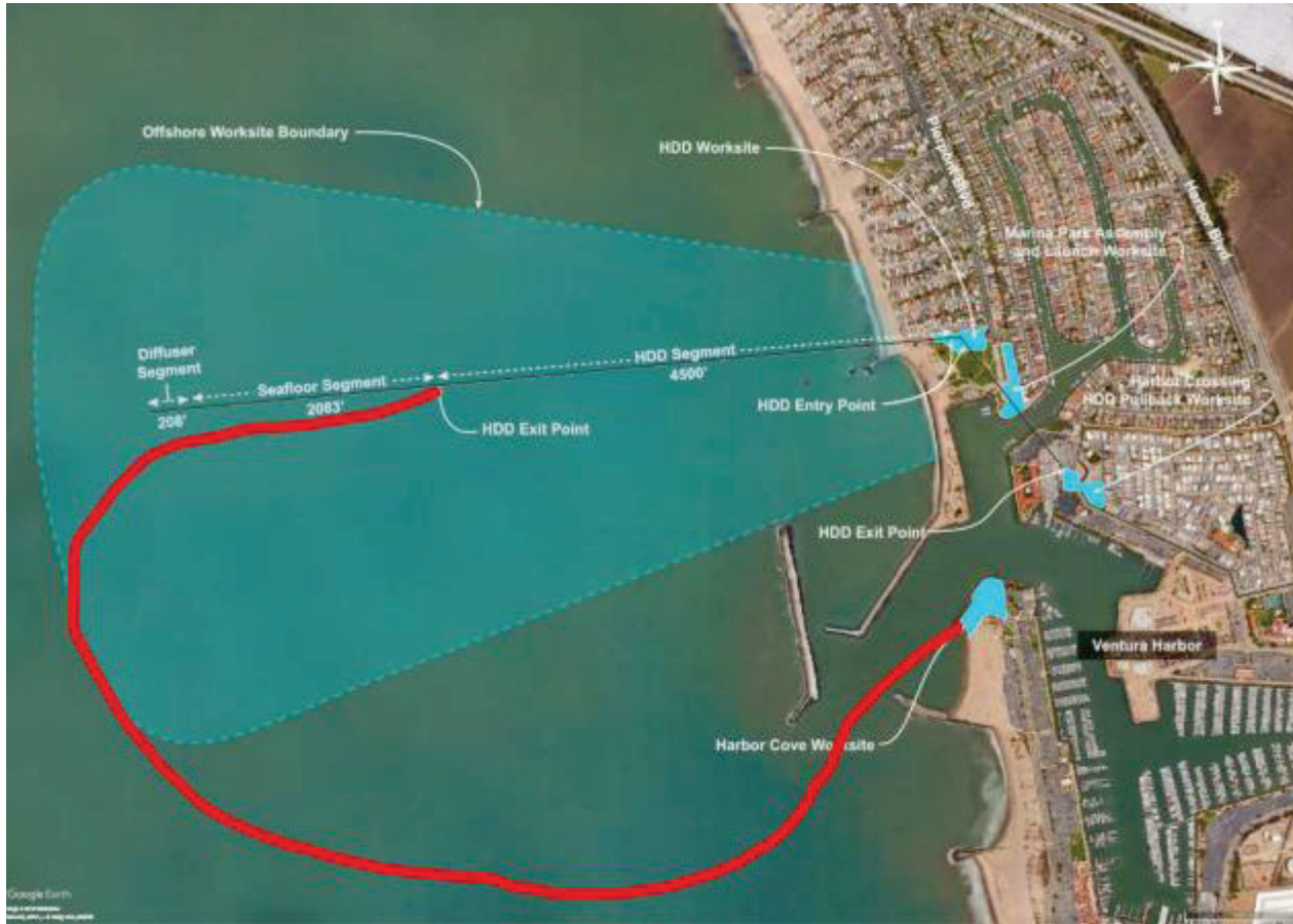
Seafloor Segment HDPE Pipeline pull-out route
