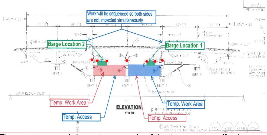
The upstream and downstream ends of the temporary cofferdams and each corner of each flexi-float barge shall be lighted at night with steady burning red lights visible at 2,000 yards by approaching vessels. Only one span will be worked on at any one time, leaving the other span available for mariners.
