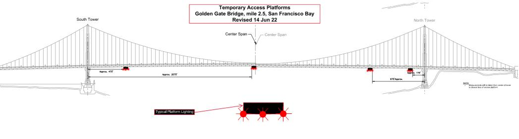
Four 54 ft wide temporary platforms are installed in the main span below low steel of the bridge, in relation to centerline of the span; two south of the north tower and two north of the south tower, reducing vertical clearance by no more than 14 feet. The upstream and downstream lower edges of the temporary platforms will be lighted at night with steady burning red lights visible at 2,000 yards by approaching vessels.
