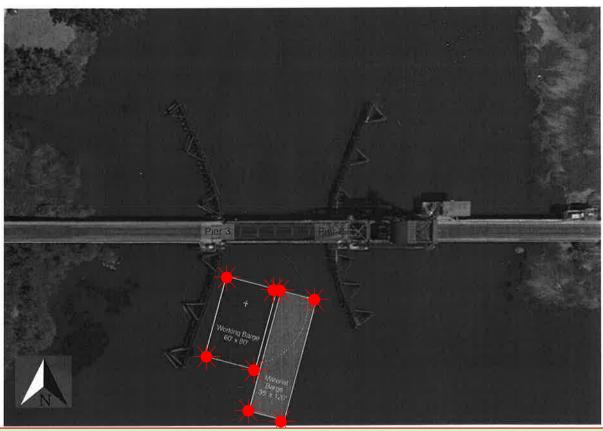
During working hours the barges will be in the main span of the bridge. The barges can be moved for navigational safety upon request with one hour advance notice. After normal working hours the barges will be moored behind the wing-walls of the pier protection system and each corner of each barge will be lighted at night with steady burning red lights.
