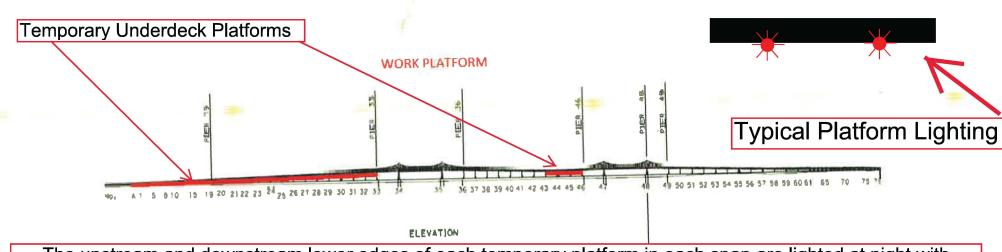
The upstream and downstream lower edges of each temporary platform in each span are lighted at night with steady burning red lights to be seen at 2,000 yards by approaching vessels. Each platform reduces vertical clearance by no more than 3 feet.
