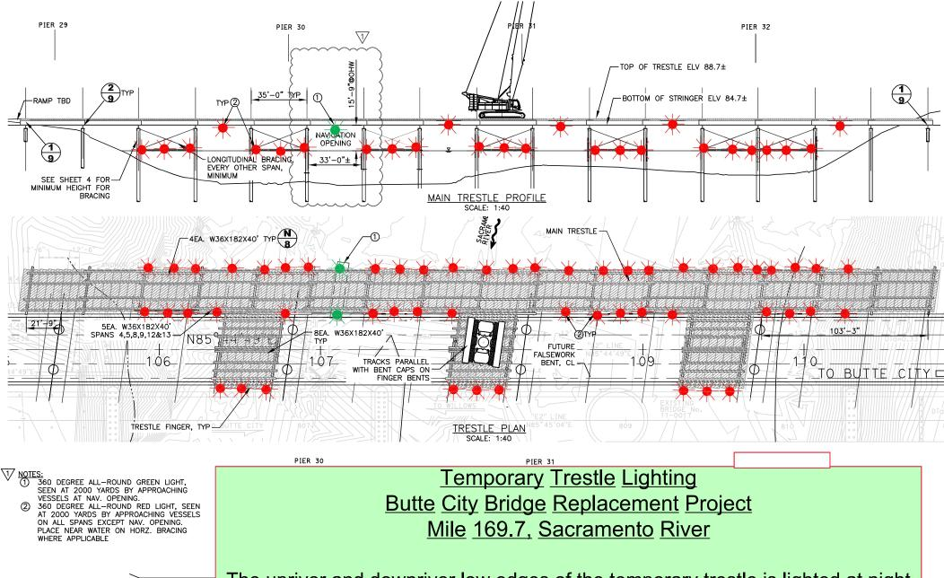
The upriver and downriver low edges of the temporary trestle is lighted at night with steady burning red lights. The recommended navigation span during the replacement bridge project has a green center channel light on the upriver and downriver portion of the temporary trestle.
