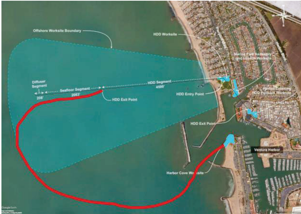
Seafloor Segment HDPE Pipeline pull-out route
