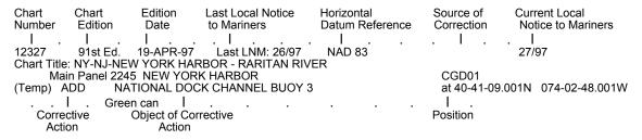
(Temp) indicates that the chart correction action is temporary in nature. Courses and bearings are given in degrees clockwise from 000 true. Bearings of light sectors are toward the light from seaward. The nominal range of lights is expressed in nautical miles (NM) unless otherwise noted.
